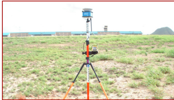
Station & Benchmarks Static Survey
